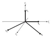
Their lengths are  $||s_1|| = \sqrt{2}$ ,  $||s_2|| = \sqrt{2}$ ,  $||s_3|| = \sqrt{3}$ , and  $||s_4|| = \sqrt{3}$  and the corresponding signal energies  $E_k = ||s_1||^2$ , k = 1, 2, 3, 4.
