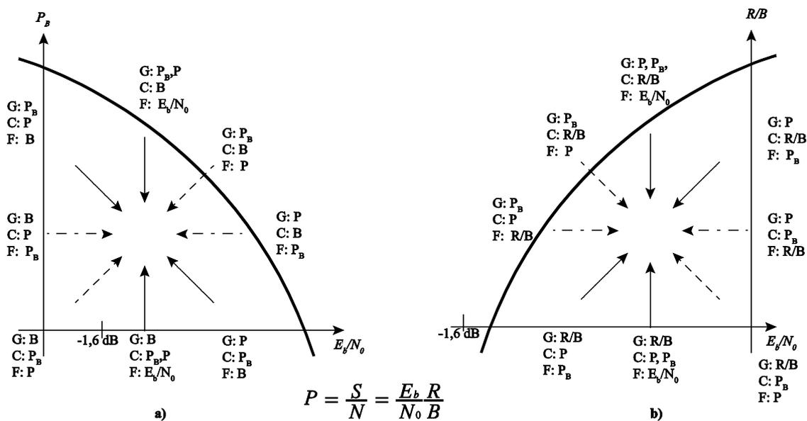
Figure 7.6 Modulation/coding trade-offs: a) Error probability plane, b) Bandwidth efficiency plane.
