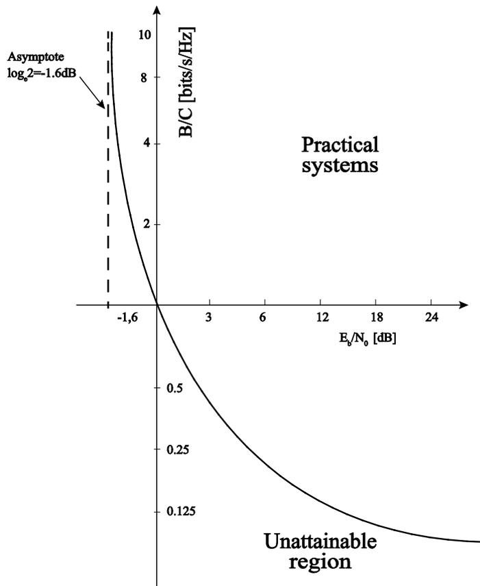
Figure 7.4 Normalized channel bandwidth versus channel  $\frac{E_b}{N_0}$ .
