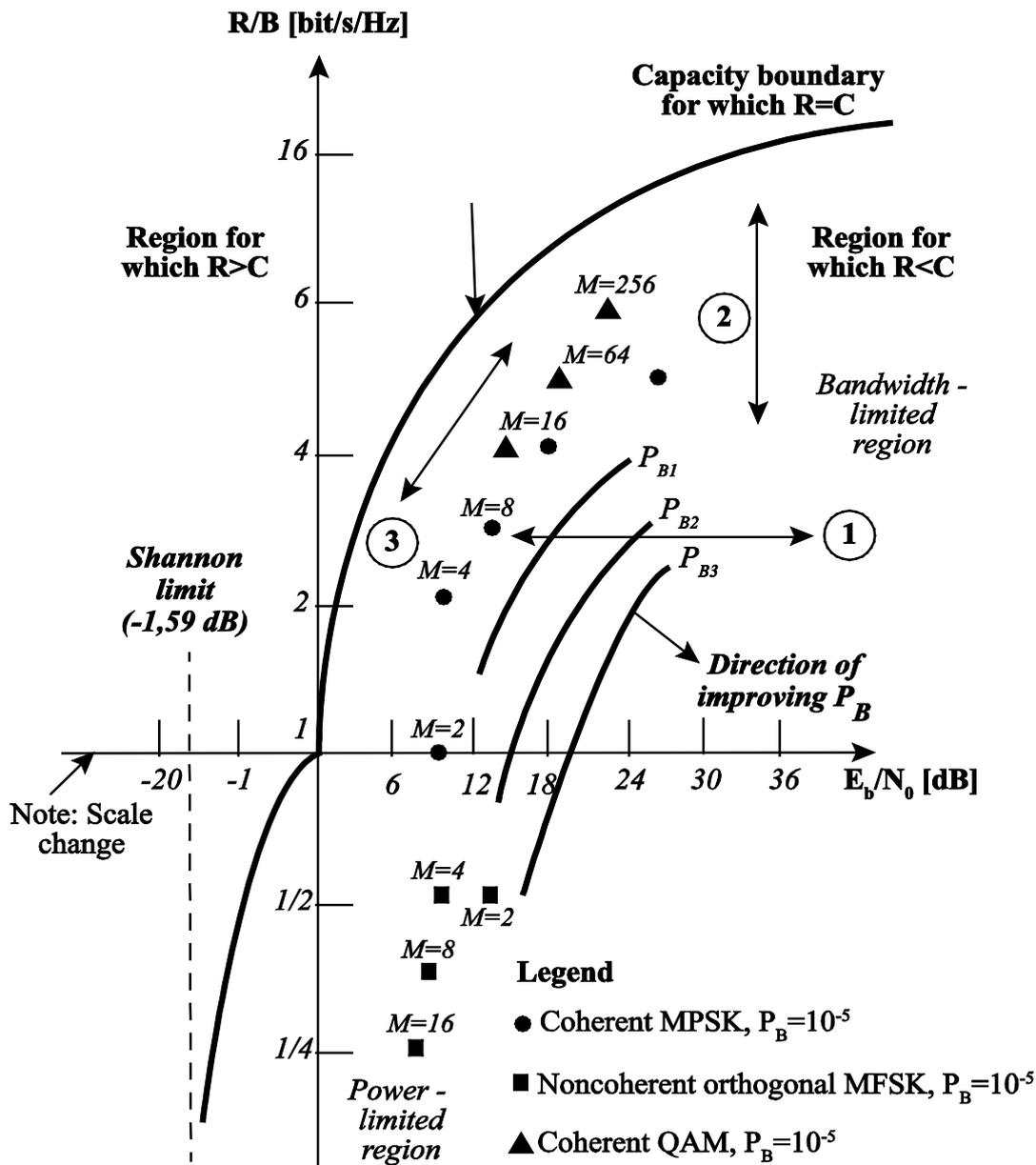
Figure 7.5 Bandwidth-efficiency plane.
