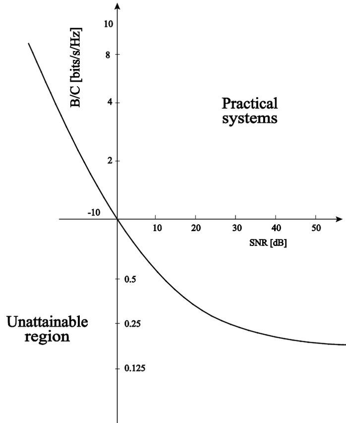
Figure 7.3 Normalized channel bandwidth versus channel SNR.
