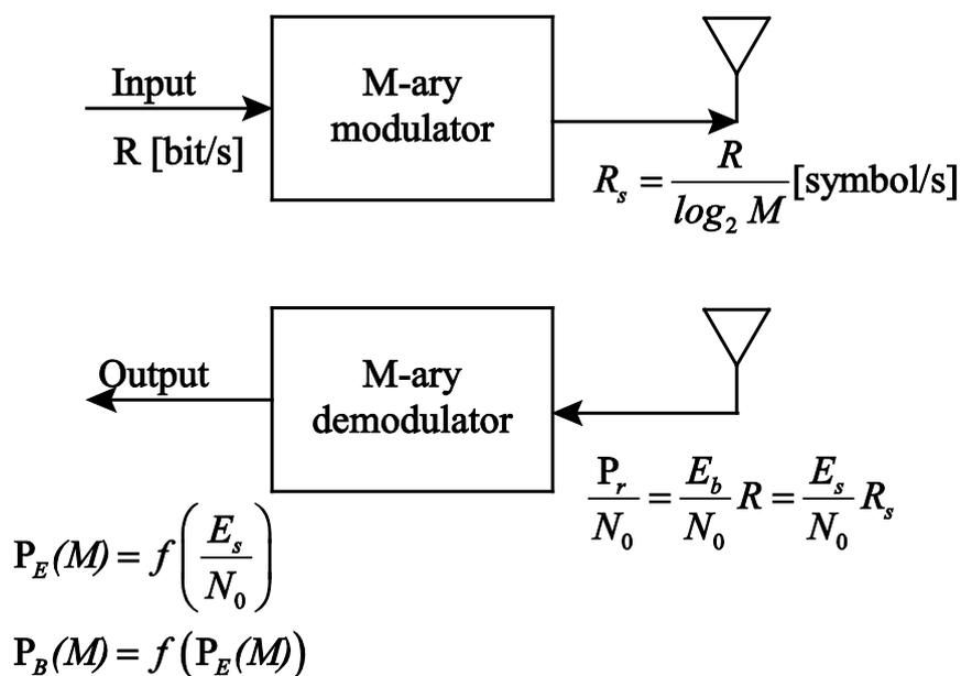
Figure 7.7 Basic modulator/demodulator (MODEM) without channel coding.
