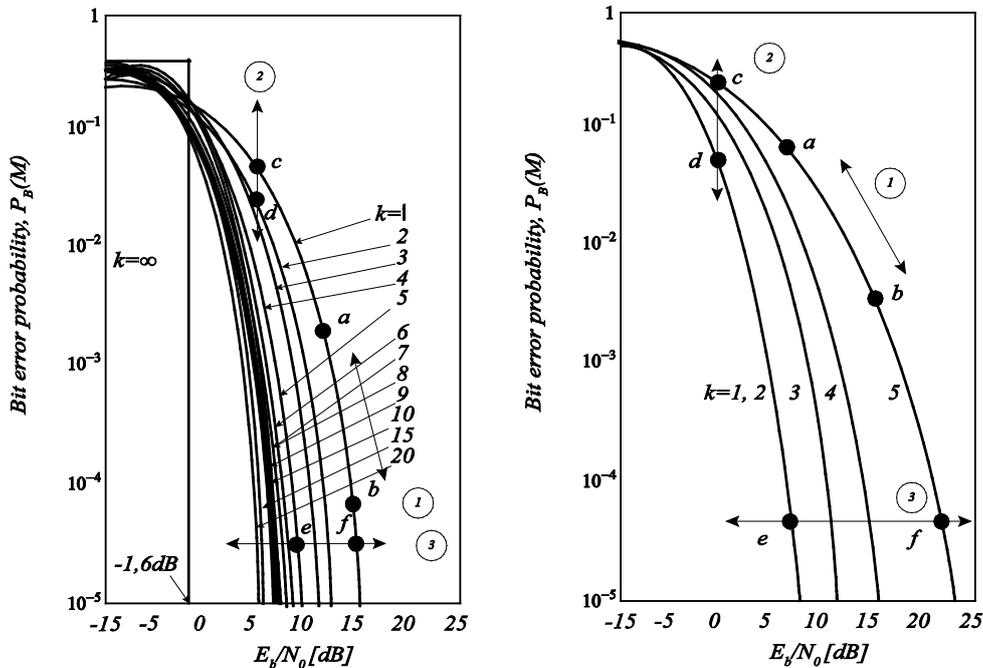
Figure 7.1 Bit error probability versus  $\frac{E_b}{N_0}$  for coherently detected M-ary signaling: a) Orthogonal signaling, b) Multiple phase signaling.
