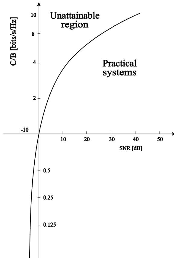
Figure 7.2 Normalized channel capacity versus channel SNR.
